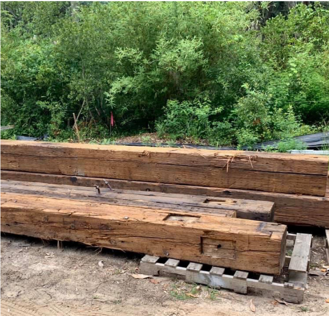
(Above) Esposito Construction transported rafters and beams from a decommissioned railroad house and carousel and refinished them.
